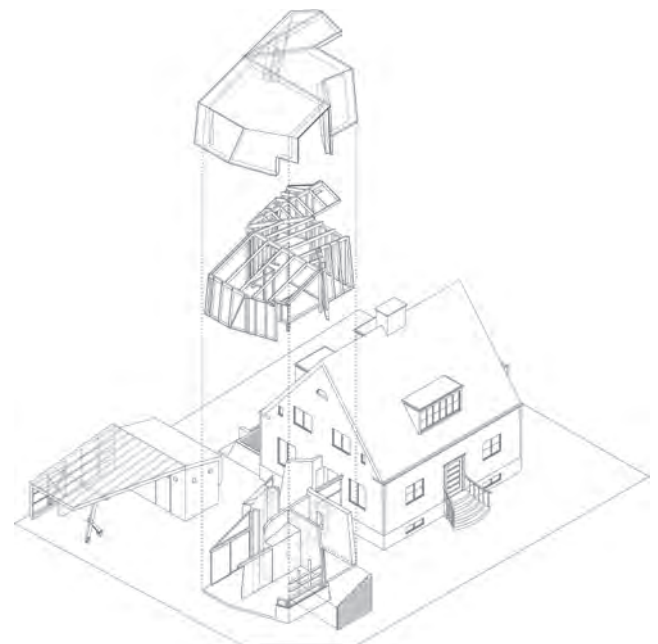
6 smogstudio建筑事务所, Unit C, 拓扑学的结构概念包含了板、墙和表皮, 瑞典洛阿, 2017/smogstudio, Unit C, the structural concept in topology conflates slab, wall, and skin, Råå, Sweden, 2017 ( 5.6图片来源/Sources: ©smogstudio )
